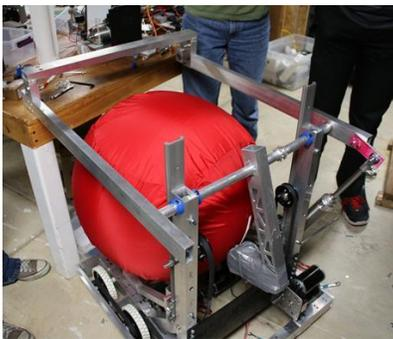
The kicker also used an aluminum foot that we curved using the CNC machine to make our design simpler and better looking than the
