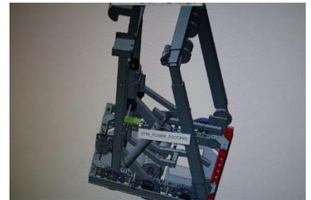
The final design that we settled on was based on our prior designs as well as the feedback that we had received on Chief Delphi and it was by far our best. We moved the pivot point of the intake mechanism to the bottom of the robot rather than the top to make extending to the desired distance easier and our mount solution stronger. We also decided to use the Igus slew rings that we had received in
