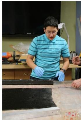
pieces of carbon fiber rectangular tubing for the “Intake”
