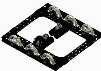
meccanums with the AndyMark chassis, but this had a number of drawbacks. First, the frame wasn't sturdy enough for mecanum wheels and because of this we couldn't maneuver like we had expected the mecanum wheels to be able to. Usually one wheel was higher off the ground than the other three and when we tried to move sideways the robot either
