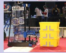
Even more exciting, during a 15 second autonomous mode (non-driver controlled) the team was able to successfully get the robot to stack the 3 yellow totes and place them in the AutoZone for an additional 20 points. This didn't work at all during the qualification rounds, but they tuned in their code and during the elimination rounds (8 rounds) it never failed! What an amazing accomplishment by the programming
