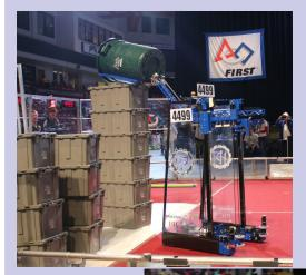
**So what did the robot have to do?** In driver operated mode, it had to stack totes up to 6 high and place a recycling container on top for points.
