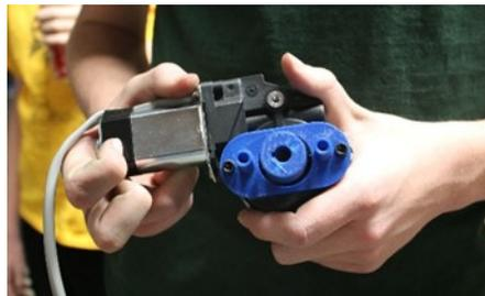
deal with the complexity of the part, the torque applied to it exceeded its capacity, and it failed. We redesigned with a metal part, and learned a valuable lesson.
