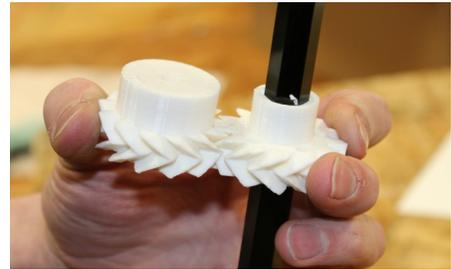
Both the Novo 1800 and Colorfabb HT filaments are co-polyester plastics and so have a low coefficient of expansion. We used these filaments to build high strength, high accuracy parts. - Pulleys, encoder cases, spacers and back of the shooter mechanism. Another advantage of the Colorfabb HT is the impressive heat resistance, as it can stand temperatures up to 100 degrees Celsius.
