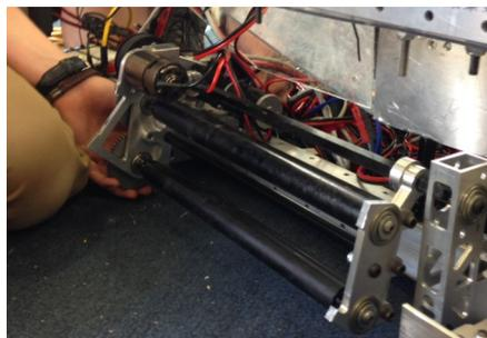
We developed a mechanism with roller bars to grab the gear after the robot drives over the top of it. The entire mecha-
