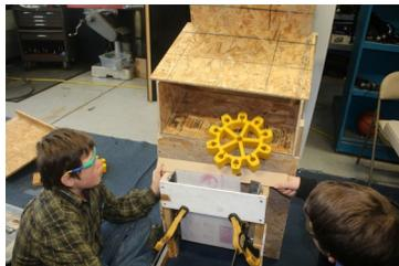
This design was promising in the preliminary stages but like the trapdoor mechanism it failed to reliably catch the gear.
