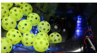
The wheel also changed from a 6" wheel to a 4" rubber wheel to give more compression to the
