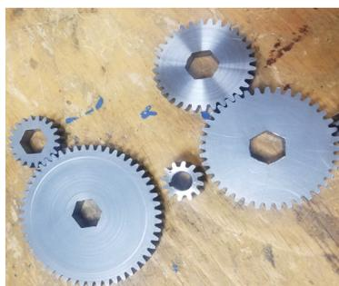
proper program. The final process to machine the gear is to lathe the gear to diameter, cut it off at the desired thickness, and then broach it to 1/2" hex.
