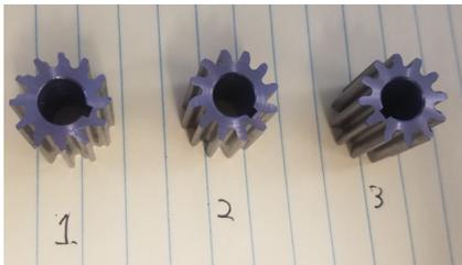
gears in FIRST robotics. To hold the involute cutter in a BT 40 collet we decided to buy an r8 arbor and lathe it down to fit in the BT 40 collet. This is due to the inexpensiveness of r8 collets and the strength of steel that it comes with. To hold the work in the 4<sup>th</sup> axis we devised a method of holding an available four jaw on the 4<sup>th</sup> axis by making
