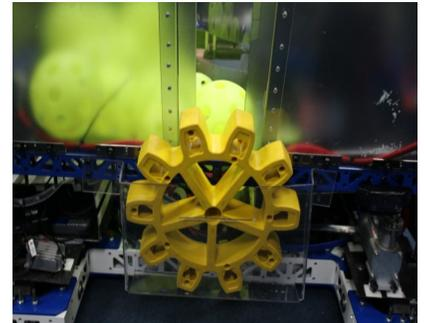
This was the mechanism that we used at the Hub City Regional. While we were able to easily deposit the gear on the spring once we had it, we were only able to catch 50% of the gears from the feeder station. Worse yet, the failures to catch actually ended with the gear inside the basin, making it illegal for us to get any others. It also interfered with the balls in the basin, impacting our ability to shoot.
