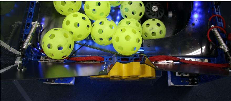
systems, the compressor and array of air tanks. Tube layout was prioritized, and we managed to avoid large curves, and have no U curves in the entire system. Channels through the chassis tubing to the piston subsystems were designated, and all the tubes were covered in nylon sheathing as to not catch. Our team learned, and put together a routing system that greatly improves to that of last year.
