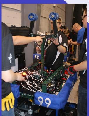
The team faced difficulty during inspection, the arm was slightly out of frame perimeter! Students and Alumni rushed to fix it. After some quick thinking, they decided to saw off part of the arm and then reattach it. After that, inspection was a breeze!
