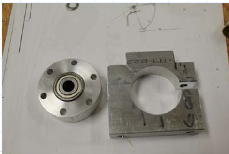
Here is the bearing and motor mount
