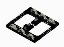
competition we used the standard AndyMark chassis with C-Channels and Toughboxes. Our team's twist on the design was our use of meccanums with the AndyMark chassis, but this had a number of drawbacks. First, the frame wasn't sturdy enough for mecanum wheels and because of this we couldn't maneuver like we had expected the mecanum wheels to be able to. Usually one wheel was higher off the ground than the other three and when we tried to move sideways the robot either
