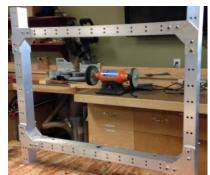
our sequences for running the CNC machine were made using the NC part of Creo provided by PTC. We used a variety of end mills to machine the beams, ranging from 3/8" roughing bits to <sup>1</sup>/4" finishing bits in order to reduce our machining time. After each of the parts for the chassis was done we sent them to another local sponsor who powdercoated them for us.
