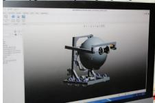
The first robot that we made used the same system that we had developed in our prototype, with wheels and a motor pulling the ball into the robot. The wheels were held out in front of the robot by an arm that
