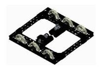
We wound up with the wheel configuration of the standard AndyMark chassis, using a live axle from the gear box for the center wheels and dead
