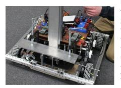
because of this we couldn't maneuver like we had expected the mecanum wheels to be able to. Usually one wheel was higher off the ground than the
