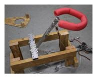
successfully in Aerial Assist. We started out trying to use pistons, but found they could be slow. We switched over to using springs (leftover from an old trampoline) and a lever arm to supply the force. To add more force, we tried combining springs and pistons, but found that the pistons actuated slowly, and our distance actually
