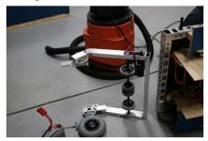
smaller wheels close to the center of the bot and two slightly larger wheels further from the center.
