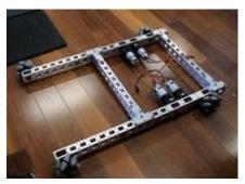
We took advantage of the space available inside the square tubing to protect the belts that connect the motors to the wheels; by running them inside the tubes we save space and protect the system. Those belts connect each Vex wheel to its own RS-775 motor with a VersaPlanetary gearbox.
