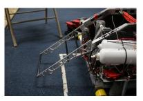
sheet metal, we designed the arms to be out of 1/4" aluminum plate for increased strength, and switched to a RS-775 with a 40:1 conversion. The
