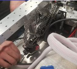
the other used wheels to pull it in a square. The two teams decided to merge their ideas, attaching wheels to the end of the square and using pneumatics to articulate the sides. The combined solution allowed for the robot to securely hold in the cube but have leeway while grabbing the cube.
