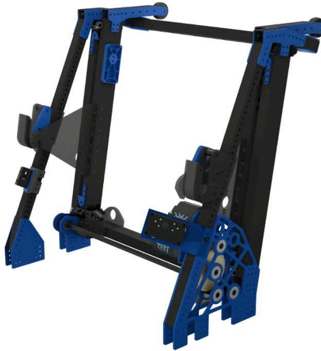
The elevator is a single stage mechanism used to climb up on the chain and subsequently raise the arm to score the trap.
