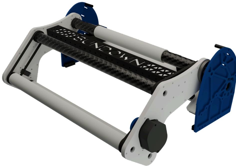
We created an over the bumper intake and rigorously spent a long time perfecting its geometry in CAD so that the intake would fit in frame without taking too much space away from other mechanisms.
