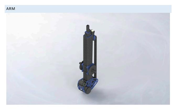
The arm contains a weighted gearbox and weight savings to maintain balance across the robot. It also has a rigid structure capable of reaching all levels and withstanding impacts from robots on the field. We also made it capable of picking up both sides of the robot.
