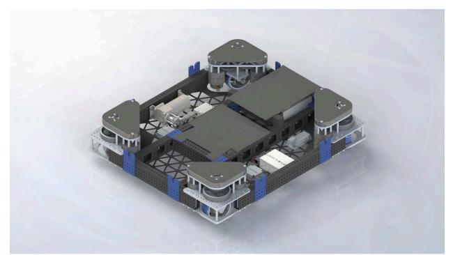
This years drive base is optimized for fast cycles and the ability to fit 3 robots on the charging station during endgame.
