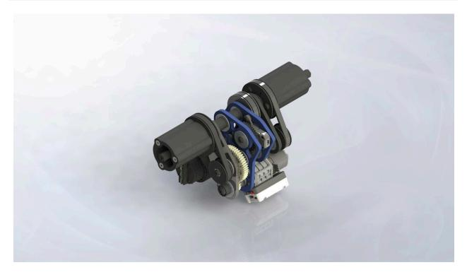
We designed this part to be compact in order to keep the weight at the end of the arm as light as possible. By minimizing the weight, we can improve the arm's maneuverability and precision. Additionally, reducing the weight at the end of the arm can help us avoid tipping over during the game.
