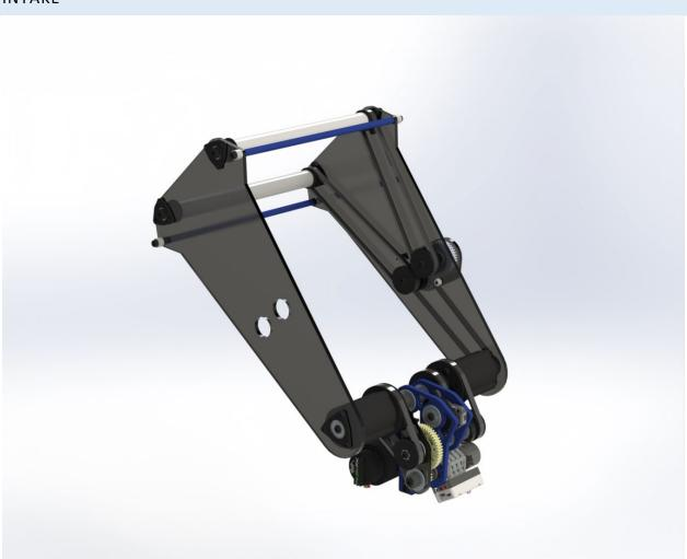
The team chose a durable and versatile design, equipped with two 12-inch rollers on the intake that can intake and place from both sides, allowing for quick and efficient collection and precise depositing of game elements from any orientation on the field.
