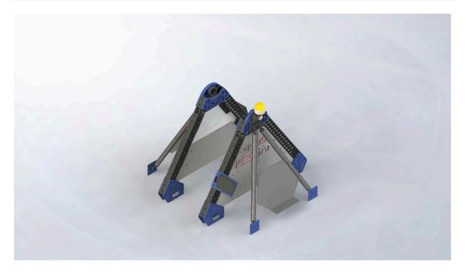
This is the support structure for the arm, which has also been designed for the ability to hotswap the arm. With multiple support structures, it is robust enough to withstand impacts from other robots and items on the field.
